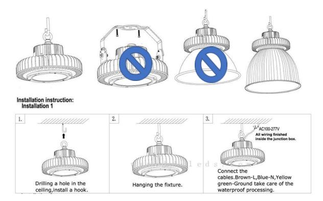
NOTE: Safety chain required for most HighBay Lighting applications and should be connected separately from hook or electrical cable.
